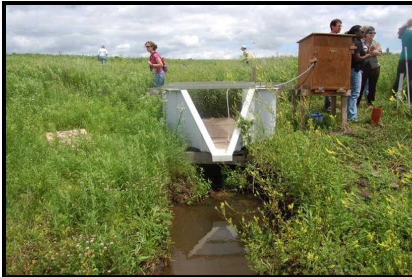
Photo 8: The stakeholder meeting concluded with a tour of the research site. A flume at the terminus of an experimental watershed is seen here. Photo courtesy of the Leopold Center for Sustainable Agriculture.
